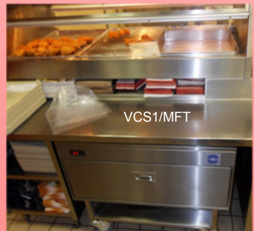
Rear Engine single drawer unit, on Mobile Frame, under hot cabinet servery
